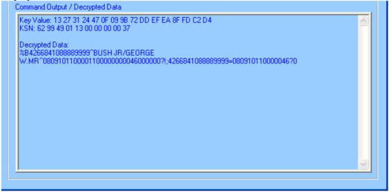
The default initial key is 0123456789ABCDEFFEDCBA9876543210. If the reader is programmed with a user-defined key, load the same key to the demo software by pressing the "Input Initial Key" button. Type the initial key in the box, and press OK when finished.
