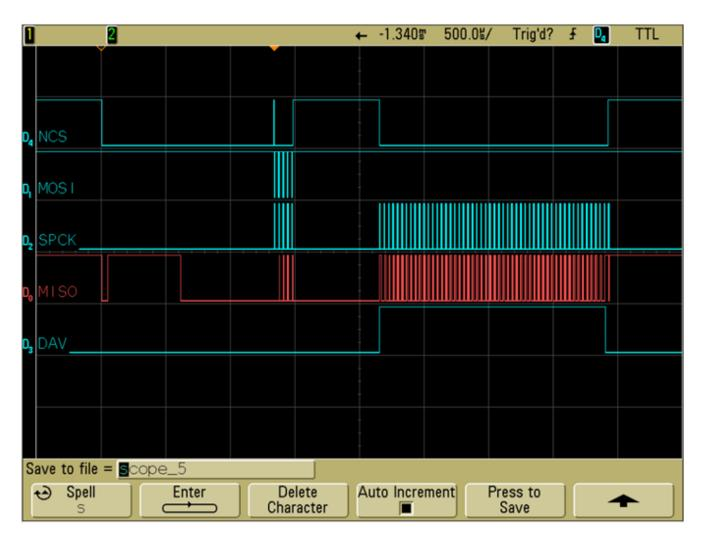
After the command is received and the response is ready, the DAV would be set to *high* for the host to receive response. After the response is received, the DAV would be *low*, indicating there is no more data to be transmitted.
