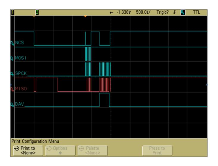
When the user swipes a card, no delay is required. Following is the waveform for MSR output:
