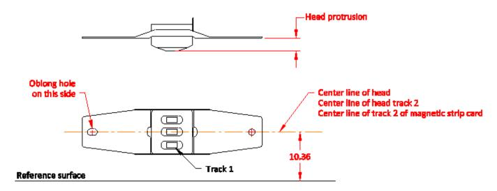
The center line of head should be parallel to the reference surface.
